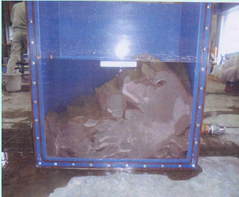
Test of material separation resistance in the water
