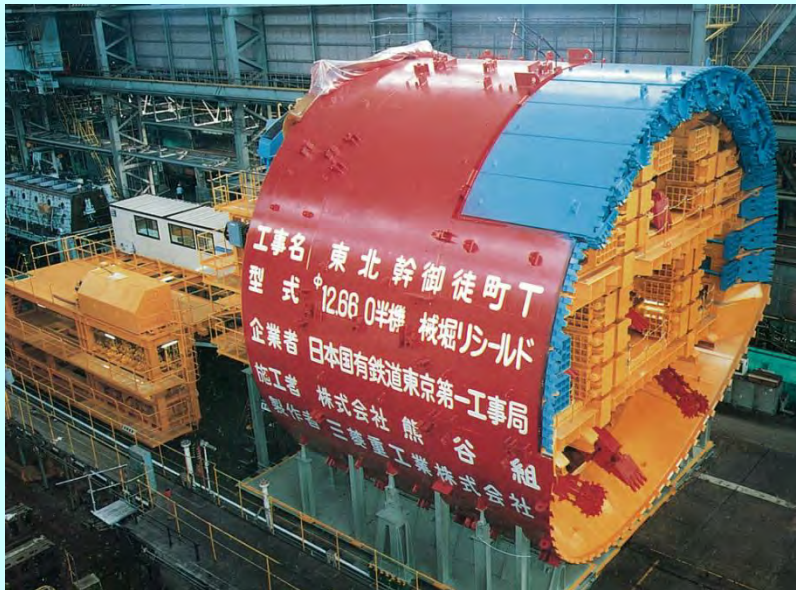
Open type shield machine (Manual excavation type)
